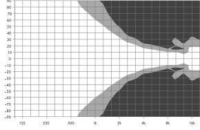
Isobar diagram T10 line source, vertical
