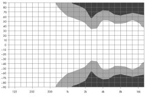
Isobar diagram T10 point source, horizontal
