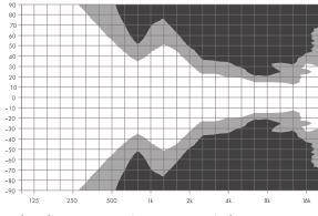
Isobar diagram T10 point source, vertical
