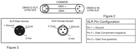
**Special Note: Line Termination.** When longer runs of cable are used, you may need to use a terminator on the last unit to avoid erratic behavior. A terminator is a 110-120 ohm 1/4 watt resistor which is connected between pins 2 and 3 of a male XLR connector (DATA + and DATA -). This unit is inserted in the female XLR connector of the last unit in your daisy chain to terminate the line. Using a cable terminator (ADJ part number Z-DMX/T) will decrease the possibilities of erratic behavior.
