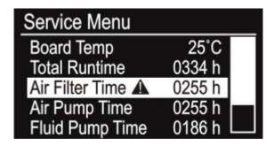
Replace component. Do not reset without replacing first. Select the correct component, press + hold 'OK' for two seconds. This will bring up a reset dialog:
