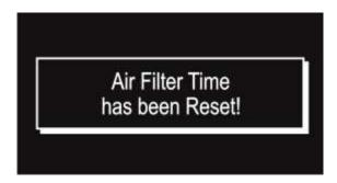
Now, the accumulated time for the concerned component is set to 0 in the service menu. The procedure is the same for the other components; Air pump & fluid pump.
