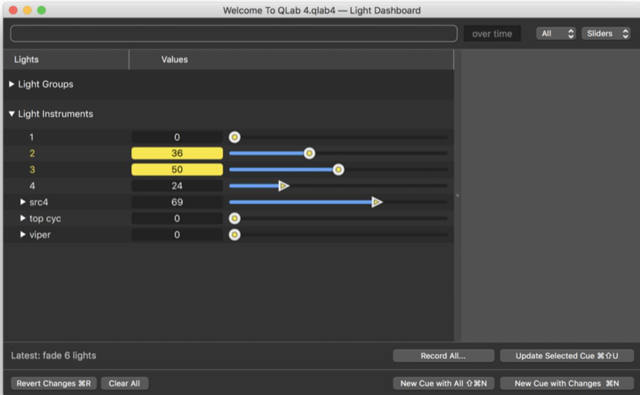
Here, a Light cue has been run which raised instrument 4 to 24 and instrument src4 to 69. Then, instrument 2 has been manually set to 36 and instrument 3 has been manually set to 50.
