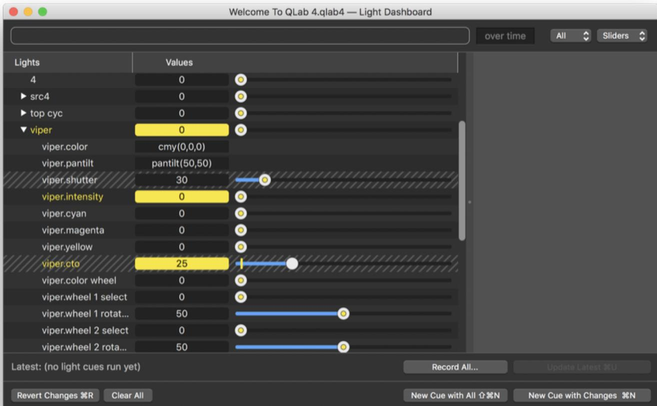
In this screen shot, two parameters of the Viper have been parked: the `shutter` parameter is parked at `30`, and the `cto` parameter is parked at `0`. The `cto` parameter has subsequently been set to `25`, and the light mark shows that the current live value of the `cto` parameter remains at `0`. All other parameters of the instrument remain unparked and can be used as normal.
