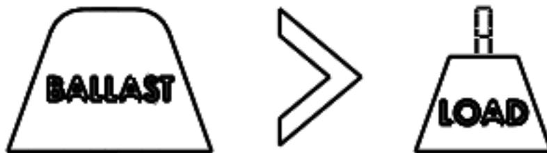
Ballast = Load x distance along boom arm x 1.2.
