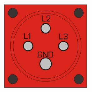
On request, unit can be equipped with CEE16/5p connector. In this case the NEUTRAL on output connector is not connected.
