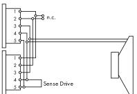
NLT4 F/M, NL4 M and EP5 connector wiring
